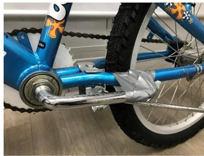
Crank remains and is taped in place
